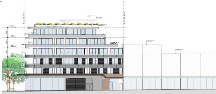
Figure 5: Extract of Eastern Elevation showing the stepping down of the building to respect the transition to lower heights in the north, as well as providing a landmark building on the south-eastern corner. (Source: PBD Architects)
