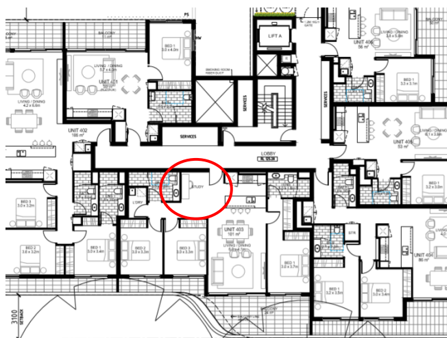
Figure 7: Extract of DA106 Revision E showing the new open study area, circled in red. (Source: PBD Architects)
